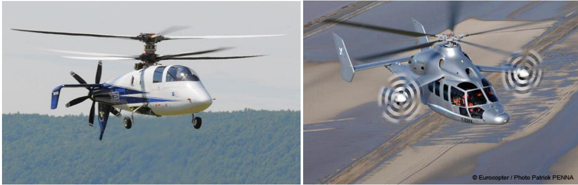
Figure 2.1: a) Sikorsky X-2 and b) Eurocopter X 3 compound helicopter technology demonstrators
